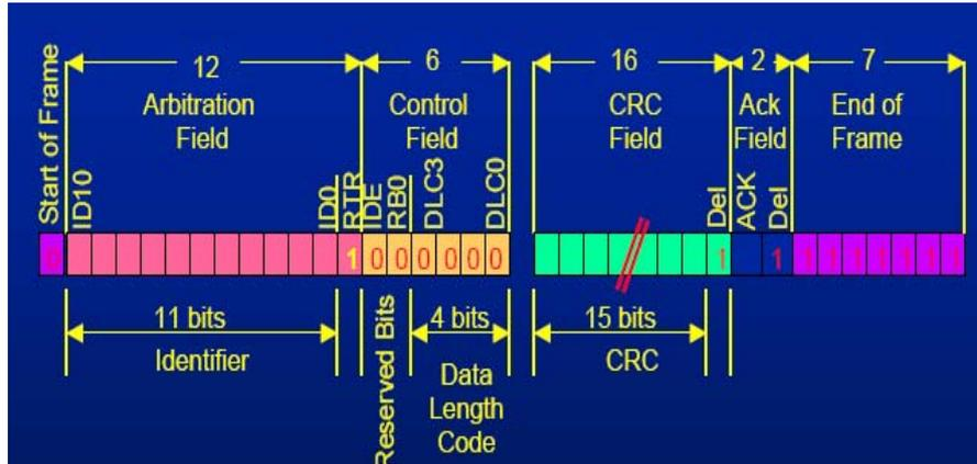
Fig4-125 - Remote Transmit Request Frame
