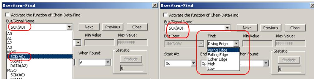
Fig 3-124: Waveform-Find Dialog Box of the SPI Signal
