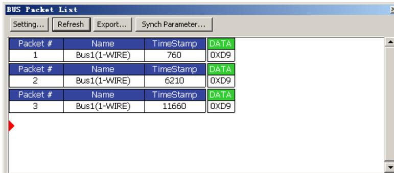
Fig4-110 - Protocol Analyzer 1-WIRE Packet List
