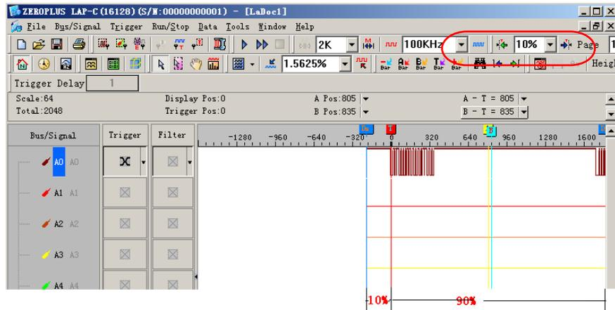
Fig 4-14 – Trigger Position 10%
