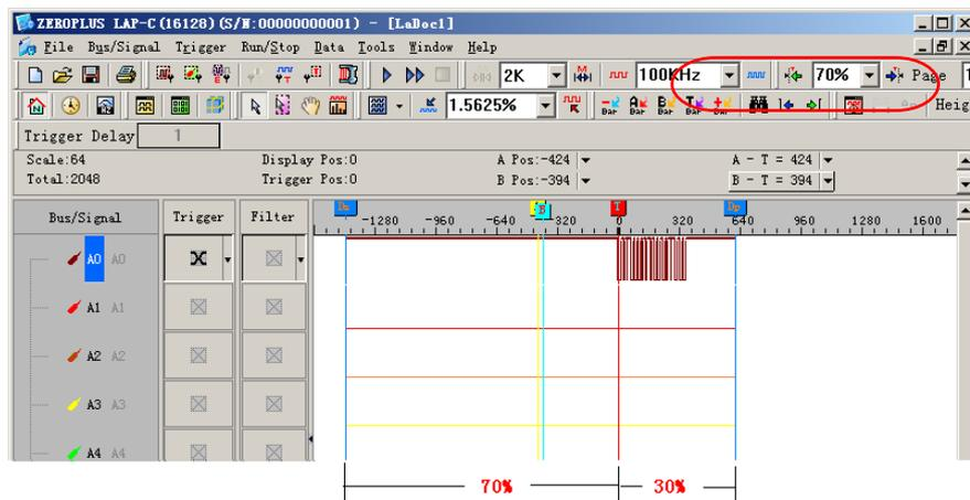
Fig 4-15 – Trigger Position 70%
