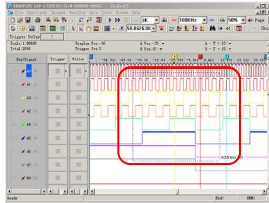
Fig 3-60: To display the Tooltip, left click and drag the mouse/point from right to left or from left to right.
