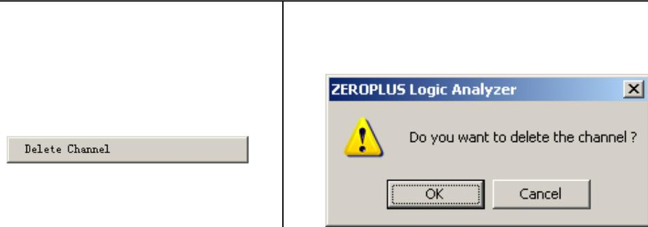
Fig3-108: Delete the selected channel in Bus/Signal column.
