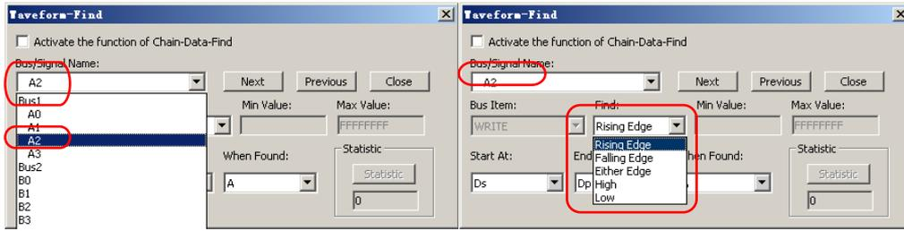
Fig 3-120: Waveform-Find Dialog Box of the IIC Signal
