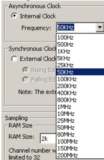
Use the pull-down menu to choose the speed of the clock on the board being tested.
