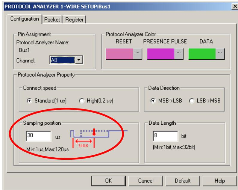
Fig4-107 - Protocol Analyzer 1-WIRE Sampling Position Setup
