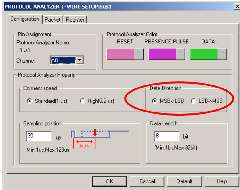
Fig4-106 - Protocol Analyzer 1-WIRE Data Direction Setup
