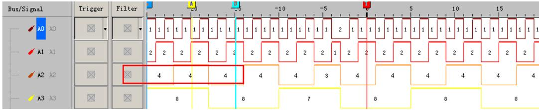
Fig4-153 - Waveforms after Filtering
