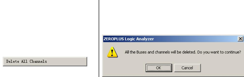
Fig 3-109: Delete all Buses and channels in Bus/Signal column.
