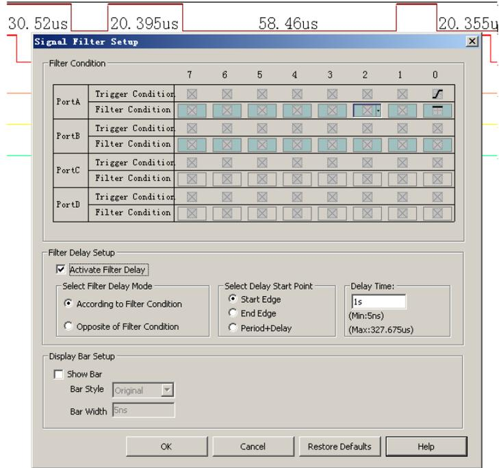
Fig 4-147 – Filter Delay Setup
