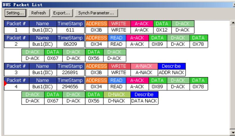
Fig4-72 - Protocol Analyzer IIC Packet List
