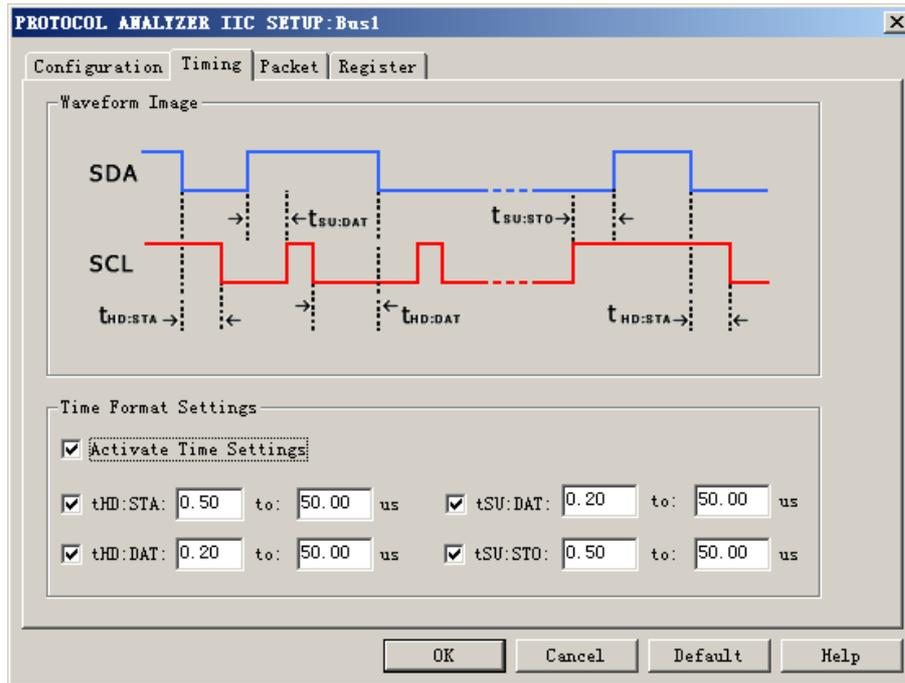
Fig 4-70 – Protocol Analyzer IIC Timing Setup
