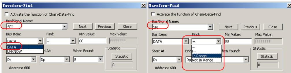
Fig 3-125: Waveform-Find Dialog Box of the Bus Item of the SPI Signal
