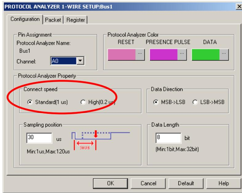
Fig4-105 - Protocol Analyzer 1-WIRE Connect Speed Setup
