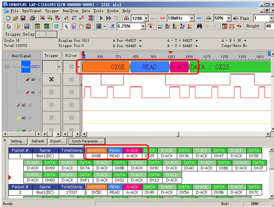
Fig 4-53 - Waveform and Packet Synchronization Interface
