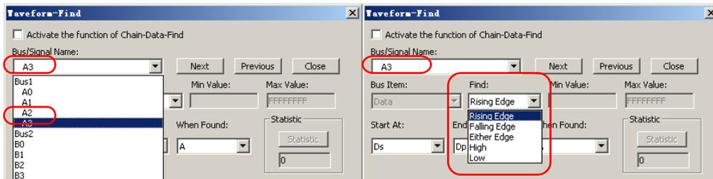
Fig 3-117: Waveform-Find Dialog Box of the Logic Signal
