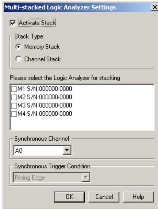
Fig 3-86: Multi-stacked Logic Analyzer Settings Dialog Box
