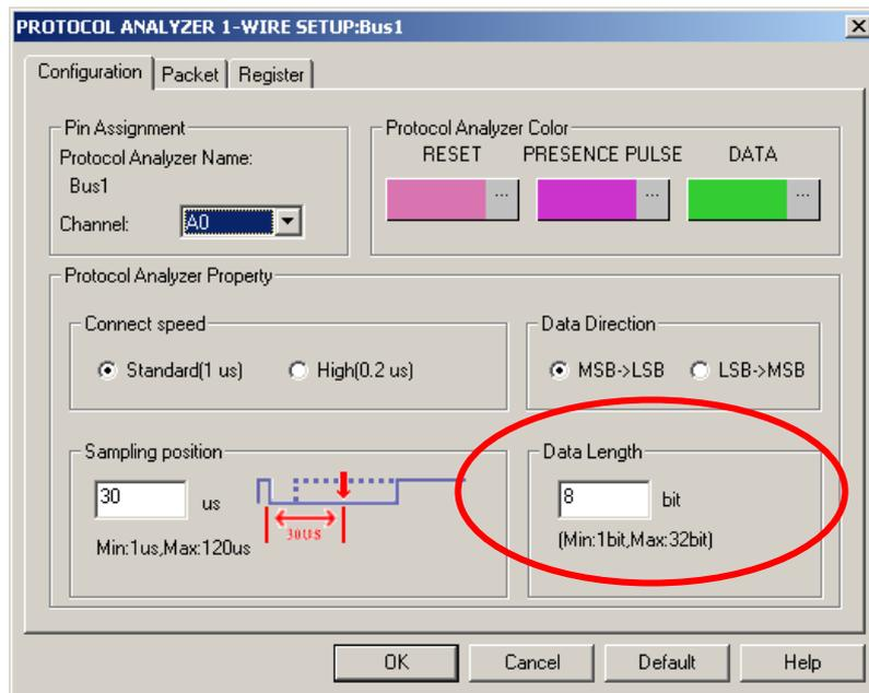
Fig4-108 - Protocol Analyzer 1-WIRE Data Length Setup
