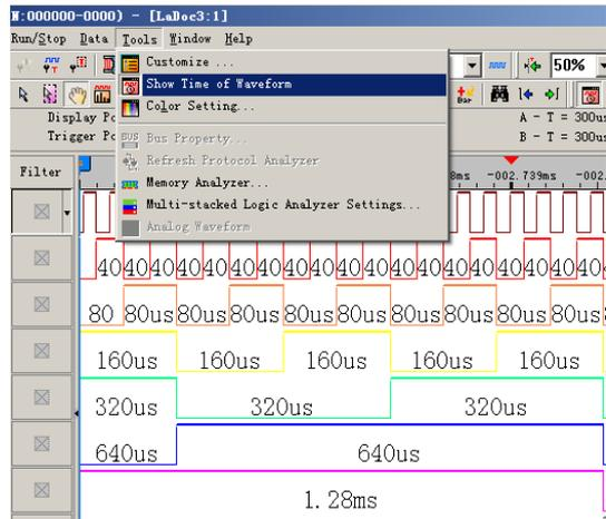
**Fig 3-80: Show Time of Waveform under Time Mode**
