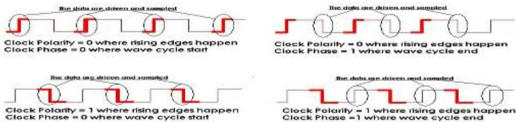
Fig 4-82 – Clock Polarity and Clock Phases
