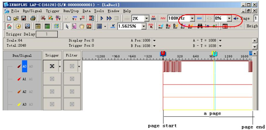
Fig 4-13 – Trigger Position 0%
