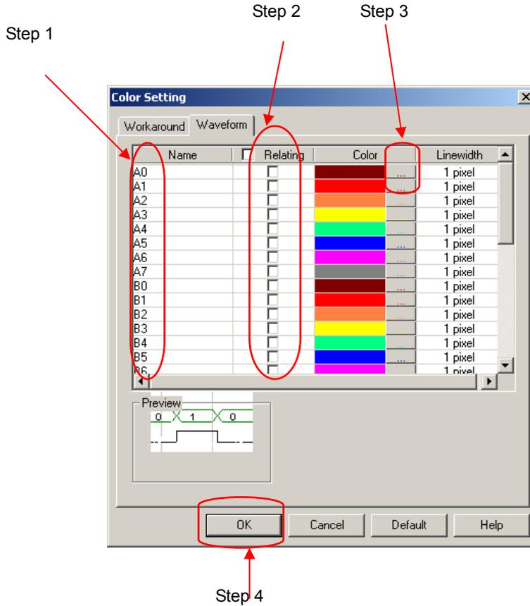
Fig 3-157: Stepwise Illustration of Changing **Waveform** Colors
