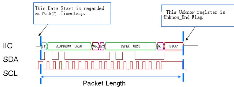
Fig4-44 - Protocol Analyzer IIC Packet Length
