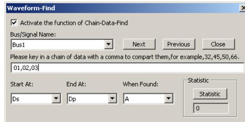
Fig 3-48: Process of Activating the Function of Chain-Data-Find
