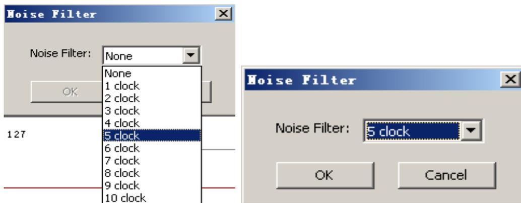
Fig4-152 - The condition of Noise Filter is 5clock.
