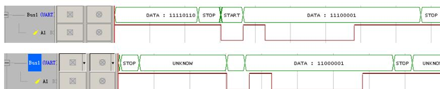
Fig 4-75 – Data Waveforms MSB->LSB and LSB->MSB
