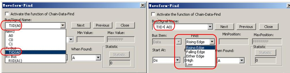
Fig 3-122: Waveform-Find Dialog Box of the UART Signal
