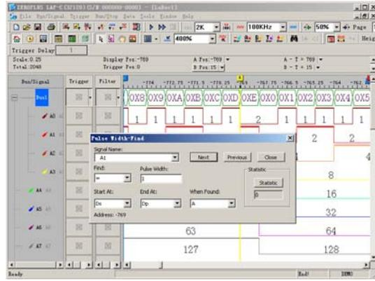
Fig 3-51: Pulse Width-Find on the Waveform Window
