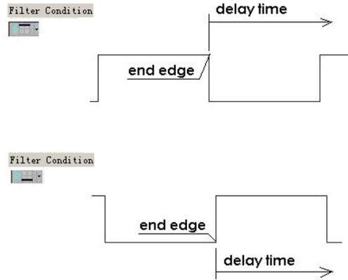
**Fig 3-25: High and Low Levels Filter Delay Setup**
