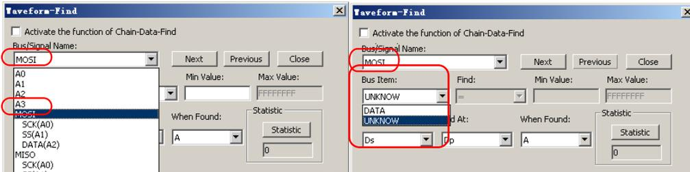
Fig 3-123: Waveform-Find Dialog Box of the Protocol Analyzer SPI
